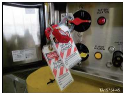
Figure 23. Battery Isolation Box – Battery isolation switch in OFF position with locks in place
